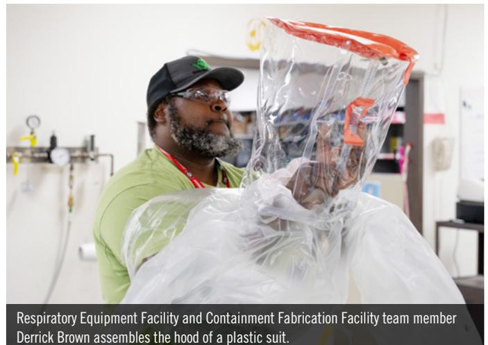
Respiratory Equipment Facility and Containment Fabrication Facility team member Derrick Brown assembles the hood of a plastic suit.
